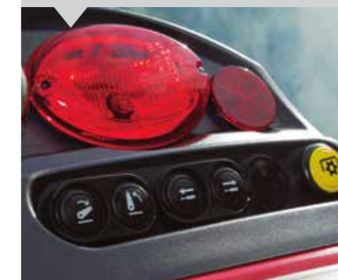
Pillar mounted PTO speed selection controls and linkage controls.
