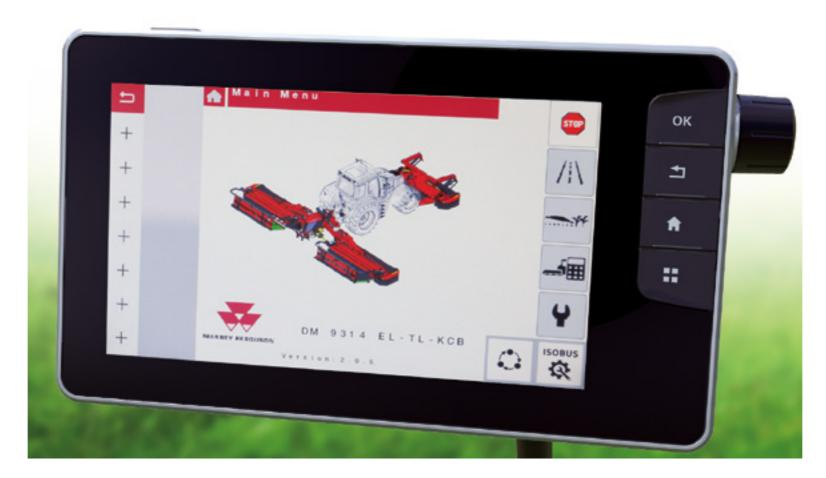
ISOBUS for total implement control – ISOBUS allows an implement manufacturer's control system to be displayed on the terminal screen, saving owners and operators time and money, with no need to install additional monitors in the cab. Simply plug the implement lead into the tractor's ISOBUS socket and the system automatically uploads the operating menus and displays on the screen. MF 6700 S ISOBUS applies to the AEF (Agricultural Industry Electronic Foundation) certification.
