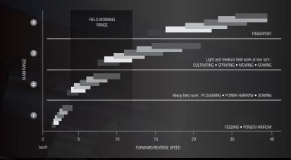
Dyna-6 offers six Dynashift changes in each range providing 24 forward and 24 reverse speeds, with an excellent overlap and a total of nine speeds in the Field Working range.
