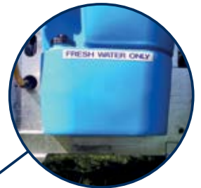
Smart Flush 105 litre on board flush tank
