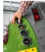
The rear power lift, PTO and one speed valve can be controlled from either rear fender.
