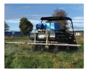
**SMART-FIT 3, 4.5 OR 6** METRE FOLDING SPRAY BOOM ELECTRIC ON/OFF KIT
