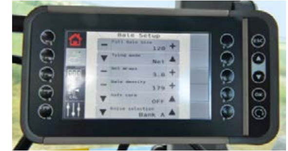
The E-Link Pro terminal gives you more functions and has an ISOBUS control unit.
