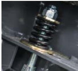
The Flexcontrol spring absorbs the load peaks from the front section of the cutting floor and therefore prevents blockages.
