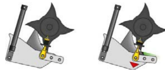
The FlexControl load relief system reliably prevents blockages.
