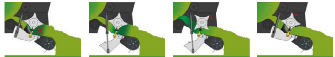
In the event of a blockage, the rear part of the cutting floor is lowered by 500 mm.
