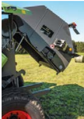
A pin on the tailgate ensures that it can be reliably closed even when used on slopes.
