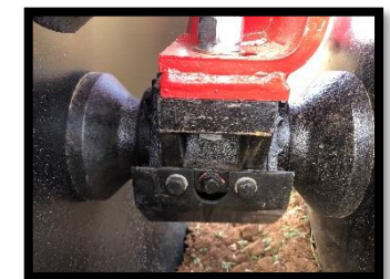
OIL BATH BEARING WITH DUO-CONE SEALS FOR EASY MAINTENANCE
