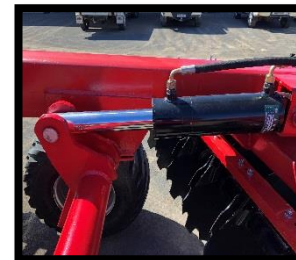
LARGE SINGLE LIFT RAM ON MAIN FRAME
