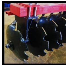
A FURROW FILLING DISC IS FITTED ON OUTSIDE OF REAR GANGS TO ENSURE A NICE, LEVEL FINISH
