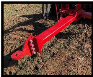
SOLID DRAW BAR WITH ADJUSTABLE HEIGHT
