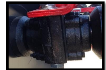
GREASE FILLED BEARING WITH NIPPLE EXTENSION FOR EASY MAINTENANCE
