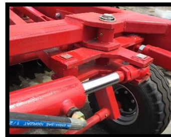
SIMPLE HYDRAULIC ADJUSTMENT OF GANG ANGLE
