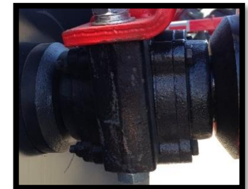
GREASE FILLED BEARING WITH NIPPLE EXTENSION FOR EASY MAINTENANCE
