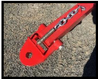
SIMPLE CHAIN AND SPRING ASSEMBLY ON HITCH ALLOWING FOR EASY HOOKUP
