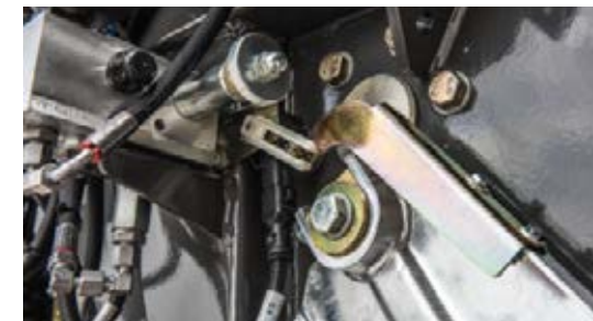
The drawbar position control ensures that the set opening angle of the pick-up is automatically sustained and controlled. This guarantees an even and constant crop flow without constriction, and clean raking even in hilly terrain.
