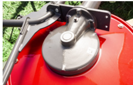
Low cost of ownership and easy maintenance thanks to the maintenance-free double-cross joints and easy access to pivot greasers and oil filled gearbox.
