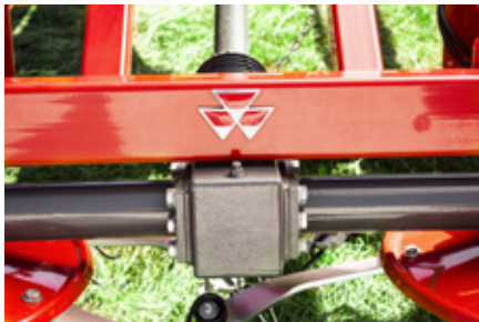
Low cost of ownership and easy maintenance thanks to the maintenance-free double-cross joints and easy access to pivot greasers and oil filled gearbox.
