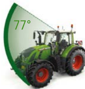
The curved windscreen of the VisioPlus cab offers a 77° viewing angle.
