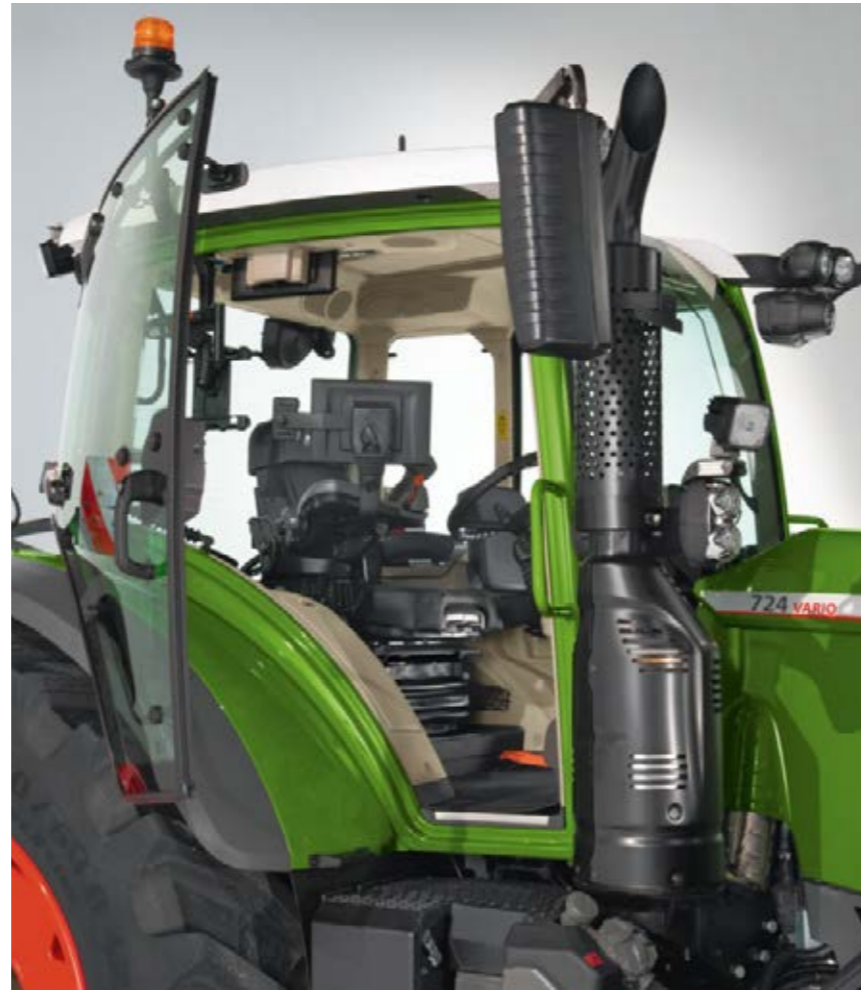
Cab configurations – choice of 3 versions: Panorama cab VisioPlus: Windscreen and right cab side do not open Panorama cab VisioPlus + right door: right door opens, windscreen does not open Standard cab VisioPlus: right door and windscreen open
