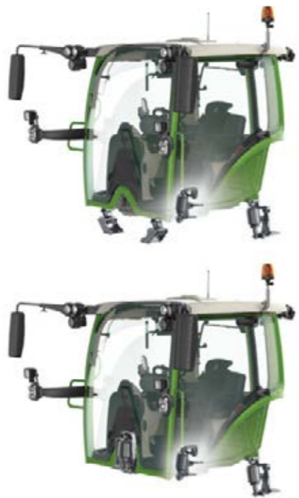
Cab suspension – choice of 2 versions: Pneumatic: cone bearing at the front, pneumatic cab suspension at the rear; 4-bearing cab, pneumatic comfort: 3-point pneumatic cab suspension (central swingarm front and 2 rear compressed air struts)
