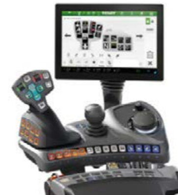
Power Setting 2 - Crossgate lever - No rocker pair (linear module) to control the hydraulic valves
