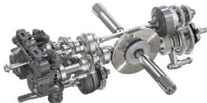
The Fendt Vario transmission is a hydrostatic-mechanical power split drive. With increasing speed, the share of the mechanical power transmitted through the planetary set increases. The hydrostats can be moved 45° and have a high operating pressure of max. 550 bar – this ensures exceptional efficiency.
