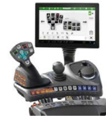
Power+ Setting 1 - Crossgate lever - One rocker pair (linear module) to control the hydraulic valves
