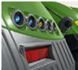
With the external valve controls, you can actuate the rear linkage, one valve and the PTO directly on the rear mudguard.
