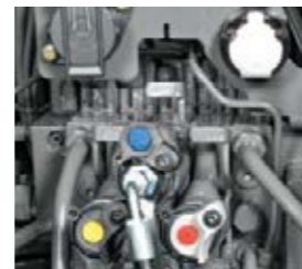
With the DCUP couplings you can couple all hydraulic valves under pressure on both sides. The pressure relief lever permits easy coupling.
