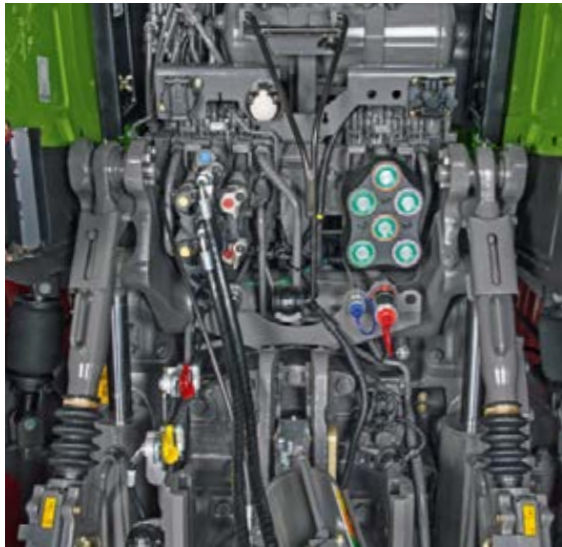
The Fendt 1000 Vario can be customised by upgrading or downgrading. The fully equipped rear area has all the connections and functions, such as Power Beyond, ISOBUS socket, rear return, PTO and rear power lift.
