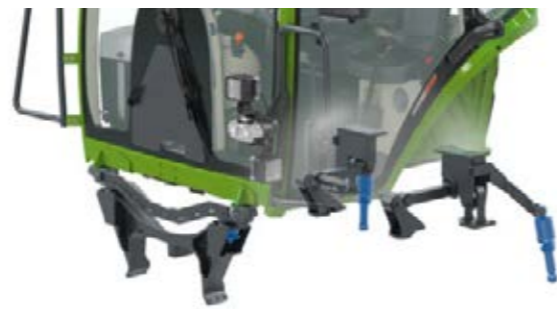
The mechanical cab suspension rests on two conical bearings at the front and on two mechanical spring elements at the rear.
