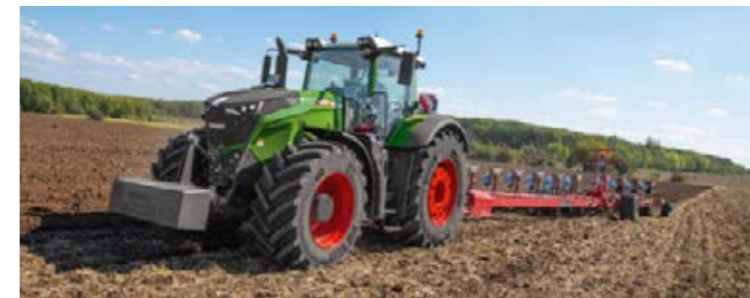
Thanks to the TMS tractor management system and the automatic maximum load control 2.0, the tractor adapts the engine speed optimally to the road speed.
