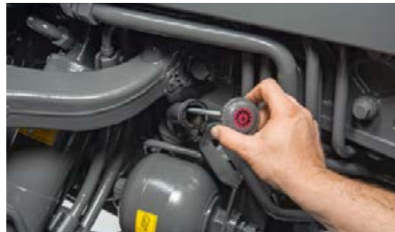
Maintenance activities, such as checking the oil level or changing the filter, are performed quickly and easily on the Fendt 1000 Vario. The engine compartment is especially easy to access thanks to the removable side panels.
