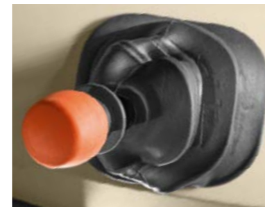
Hand brake assistant in automatic position: The hand brake is automatically activated.
