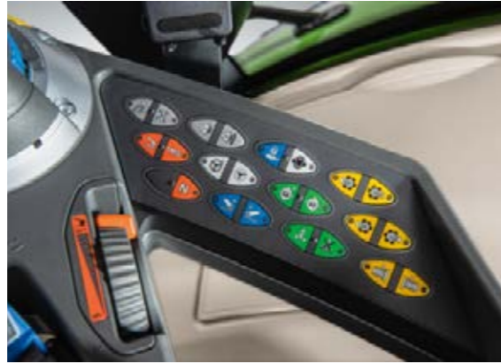
All the controls are arranged in a simple and clear layout on the backlit membrane keypad.
