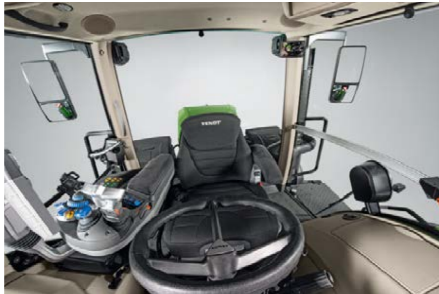
For use with reverse drive control, just rotate the operator platform a full 180°. You can then use all your controls in reverse as easily as you do in forwards mode. Despite the reversing driver station, passengers do not have to do without the comfort seat.
