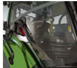
The 220° windscreen wiper on the right cab window ensures the best view to the right, even under the toughest conditions.
