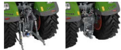
Rear power lift with quick arresters and side support
