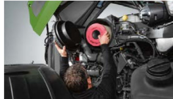
The level of dirt on the air filters is shown on the Variotermin. The engine compartment is very accessible, with removable side panels.
