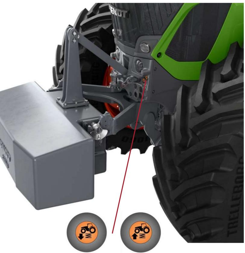
For external operation, there are buttons on the front panel.
