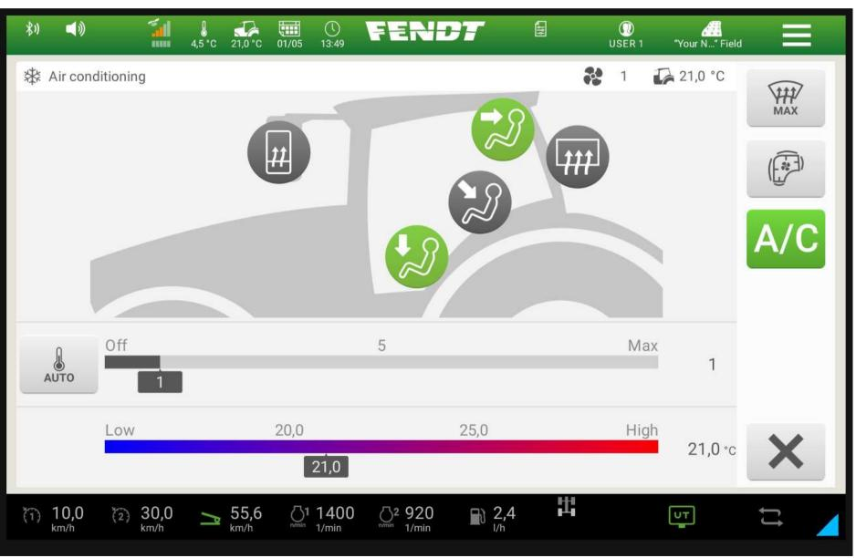
+ No need to reach up to the headliner thanks to central control on the armrest
