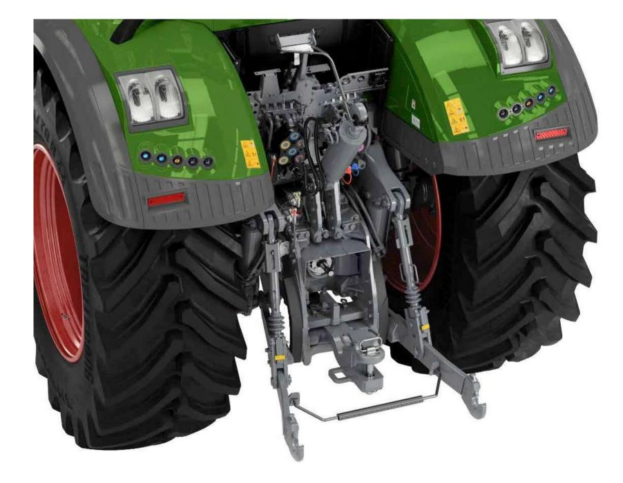
Rear linkage with quick-release hooks and rub blocks (AU)
