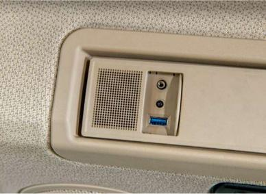
Connection of external audio sources via Bluetooth or cablebased via USB or AUX-IN connection
