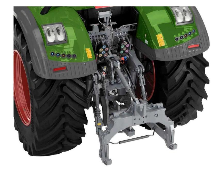
Rear linkage with ball ends and rub blocks
