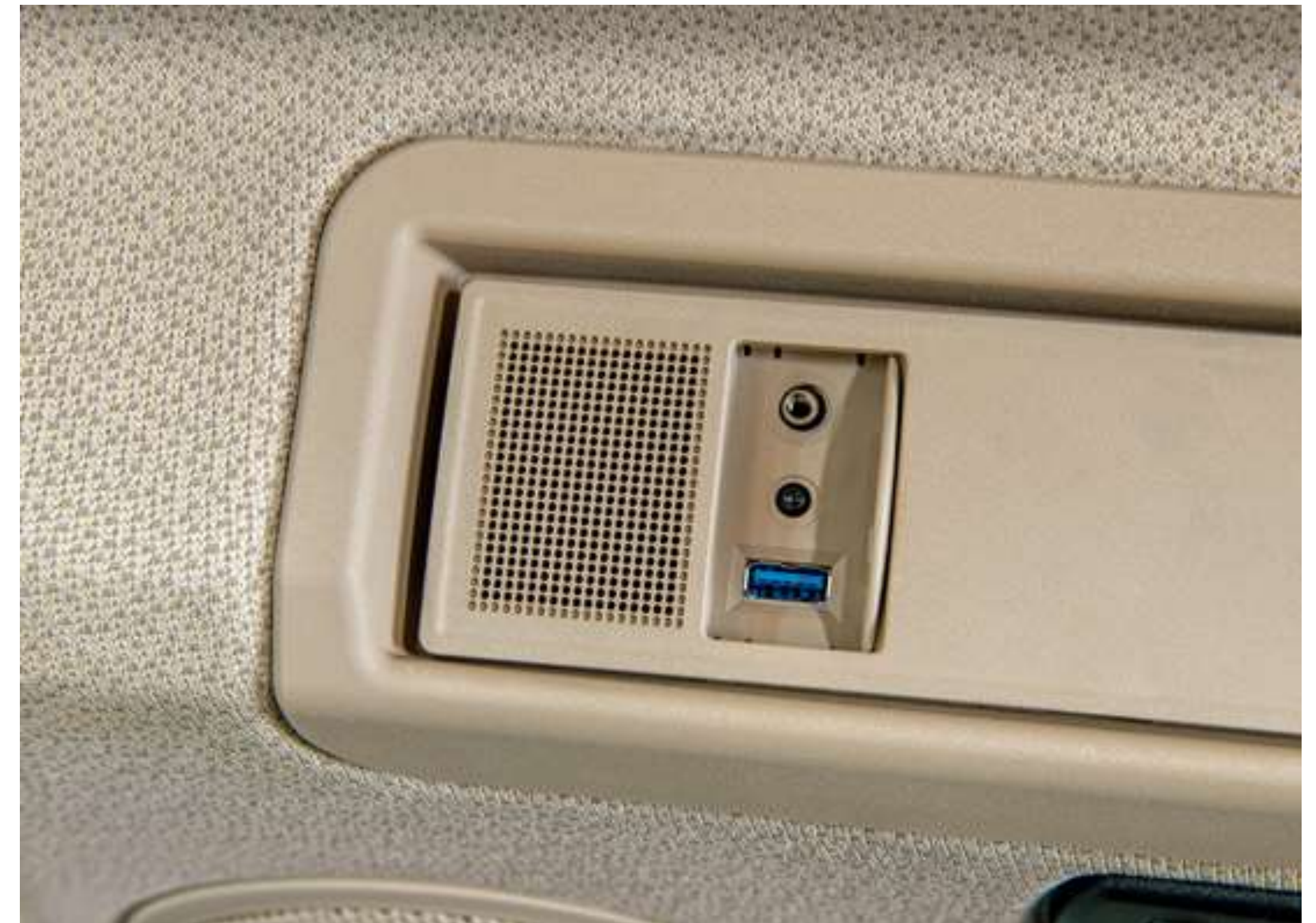
Connection of external audio sources via Bluetooth or cable-based via USB or AUX-IN connection
